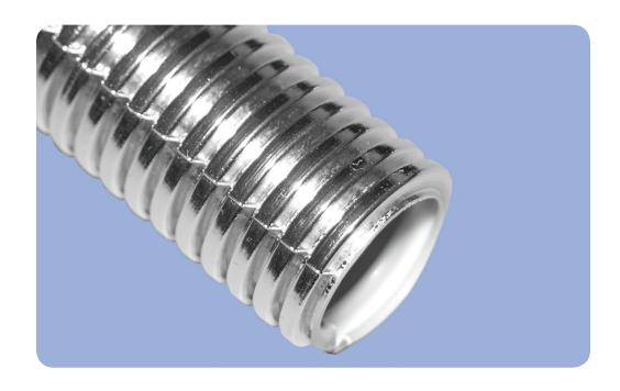
ConvoShield® AL is a reflective convolute sleeve designed to provide thermal protection for components in radiant heat environments. Composed of a high temperature nylon 4,6 polymer base substrate and a highly reflective coating, ConvoShield AL provides protection for wires, cables and hoses in applications that have radiant heat source temperatures as high as +538°C (+1000°F).
