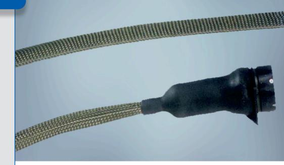
**Expando**<sup>®</sup> **HTNS-LA/HO** is a thin wall braided sleeve manufactured from Nomex<sup>®</sup>. Its highly expandable structure allows easy installation over long lengths even after the fitting of end connectors with a limited range of product sizes.
