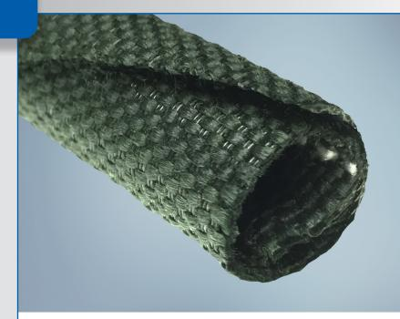
**ROUNDIT**<sup>®</sup> **2000 NX** is a woven combination of Nomex<sup>®</sup> and PPS (polyphenylene sulfide). The Nomex<sup>®</sup>/PPS blend in a flat weave construction gives ROUNDIT 2000 NX a rugged yet smooth texture and appearance for high temperature bundling and abrasion resistance. This product is rated to +200°C (+392°F) and is non-halogenated.
