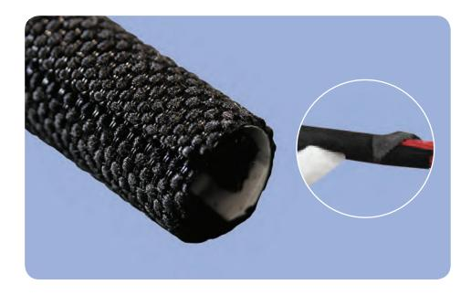
**ROUNDIT® 2000 ST** is a self-closing oversleeve designed to provide mechanical protection. ROUNDIT 2000 ST is made out of a woven substrate of monofilament and multifilament polyester yarns equipped with an adhesive tape. This unique design gives the adhesive tape the double advantage of holding the sleeve in place on the application and being a secure closing system.
