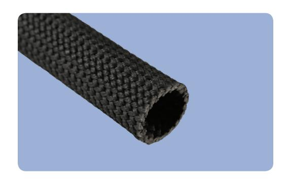
**ThermoJacket**® **B** is a coated sleeve designed to provide superior insulation protection for Exhaust Gas Recirculation (EGR) tubes. The sleeve easily withstands 400 hour soaks at +370°C (+698°F) with no discoloration of the coating. As an insulator, ThermoJacket B is used to provide maximum fuel efficiency and lowered emissions.
